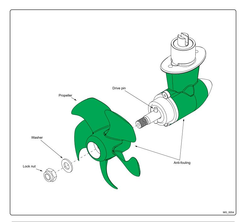
Propeller Installation MC\_0016
