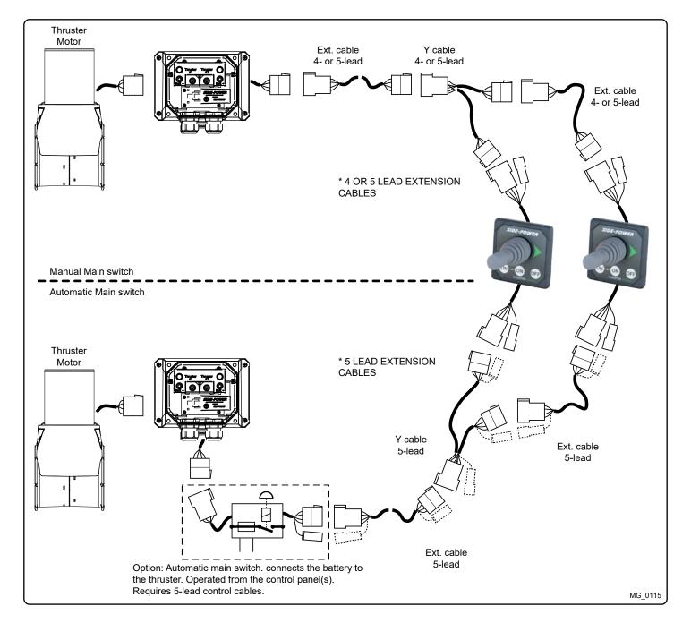
Control Panel Cable Installation
